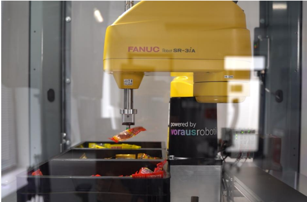
Figure 4: Pick-and-place cell with robot, conveyor belt, three boxes, and suction gripper
