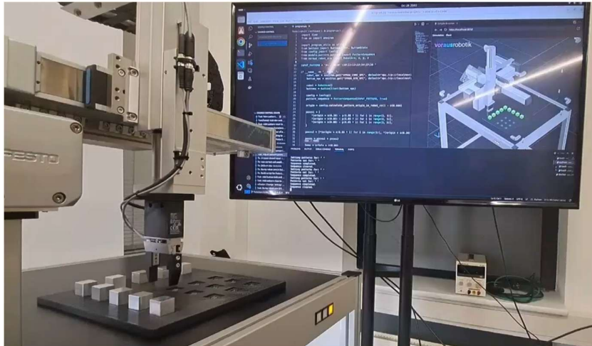
Figure 14: Individual kinematics including automatically tested control code – real plant and simulation
